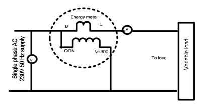
**APPARATUS USED**: one single phase energy meter (5A, 230V), one ammeter (0-5A),
